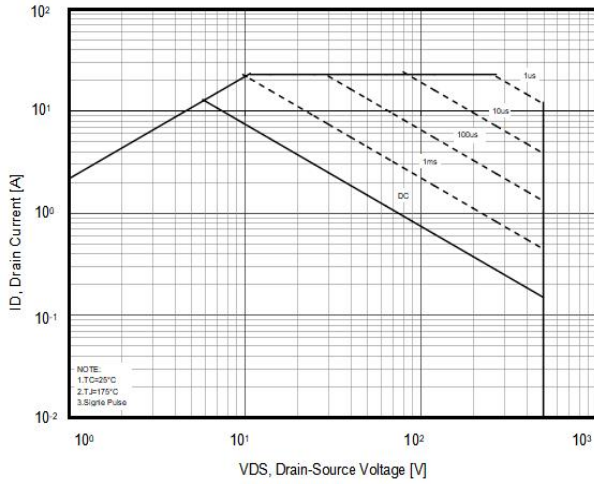
Figure1. Safe operating area
